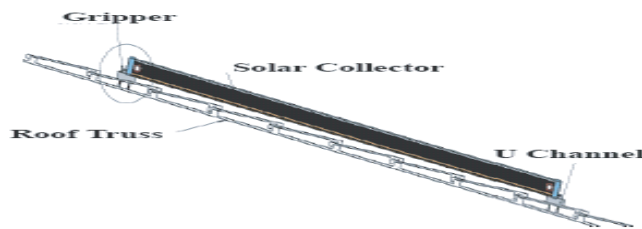
Figure #1, Flush mounted collector
