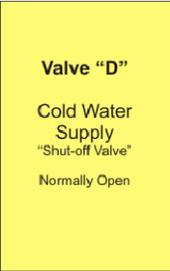
**Valve “D”** - this label is affixed to the cold water supply, “shut-off” valve.
