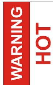
**WARNING / HOT** – labels are affixed to the collector return line at the drainback reservoir, the hot water supply line from the water storage tank and on all system components that could present a safety hazard due to high temperatures.
