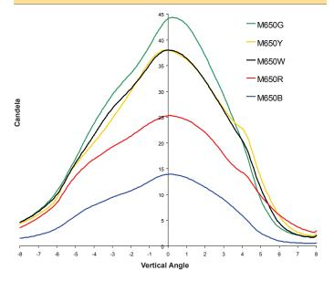
Note: Peak IALA intensity dependant on location. Plot based on equatorial location of 12-hour night duration and 21% duty cycle flash code.
