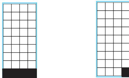
**Example of full-cell shading that can reduce PV module power to zero**
