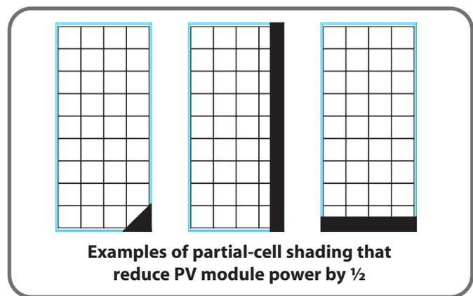
Partial-shading even one cell of a 36-cell module, such as the KD135SX, will reduce its power output. Because all cells are connected in a series string, the weakest cell will bring the others down to its reduced power level. Therefore, whether 1/2 of one cell is shaded, or 1/2 a row of cells is shaded as shown above, the power decrease will be the same and proportional to the percentage of area shaded, in this case 50%.
