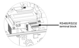
Figure 37: The RS485/RS232 terminal block
