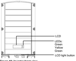
Figure 10: Inverter front view
