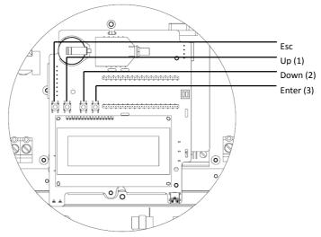
Figure 31: LCD internal user buttons
