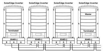
Figure 39: Connecting the Inverters in a Chain
