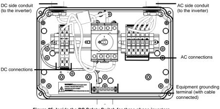
Figure 25: Inside the DC Safety Switch for three phase inverters
