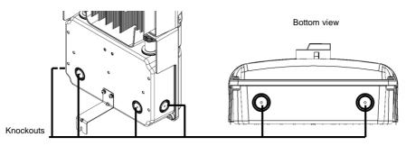
Figure 12: Safety Switch knockouts
