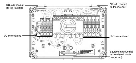
Figure 22: Inside the AC/DC Safety Switch for single phase 7.6-11.4 kW inverters
