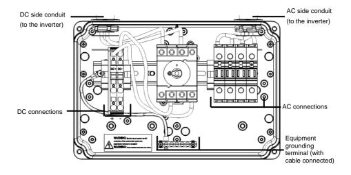
Figure 23: Inside the DC Safety Switch for single phase 7.6-11.4 kW
