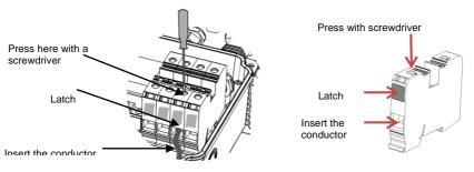
Figure 27: AC Spring-clamp terminal - single phase 7.6-11.4 kW inverter
