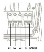
Figure 61: Three phase inverter AC terminals
