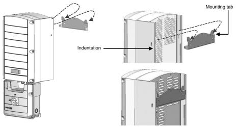
Figure 16: Hanging the inverter on the bracket - Type 2
