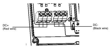
Figure 58: Single phase 7.6-11.4 kW and three phase inverter DC terminals
