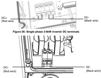
Figure 57: Single phase 7.6-11.4 kW and three phase inverter DC terminals
