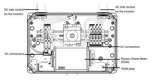
Figure 21: Inside the DC Safety Switch for single phase 3-6kW inverters with a built-in revenue grade meter (RGM)
