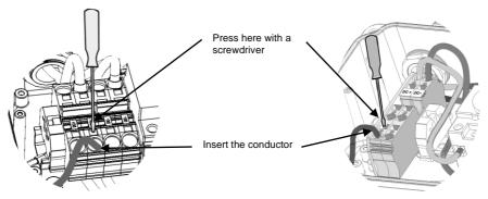
Figure 30: DC Spring-clamp terminal examples - single phase 7-11.4 kW inverter
