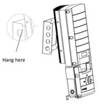
Figure 15: Hanging the inverter on the bracket - Type 1
