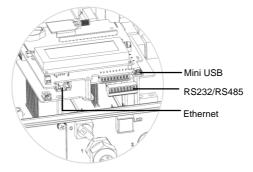
Figure 33: Internal connectors
