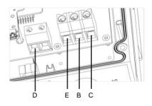
Figure 60: Single phase inverter AC terminals
