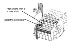
Figure 29: DC Spring-clamp terminal - three phase inverter
