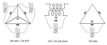
Figure 1: Auto-detected AC grids supported by SolarEdge single phase
