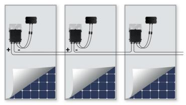
Figure 7: Power optimizers connected in series
