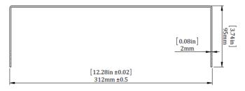
Figure 50: Three phase inverter mounting bracket
