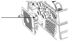
Figure 54: Fan connector
