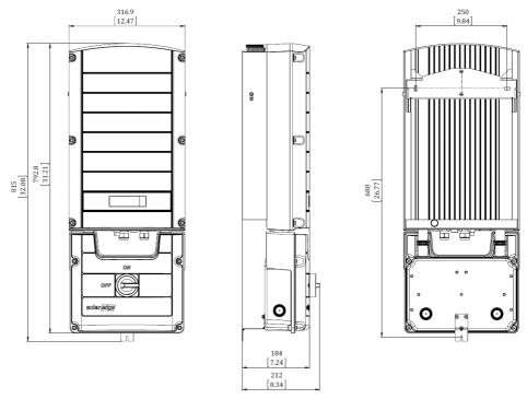
Figure 45: Single phase 3-6kW inverter with brackets - front, side and rear views
