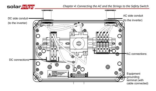
Figure 20: Inside the DC Safety Switch for single phase 3-6kW inverters
