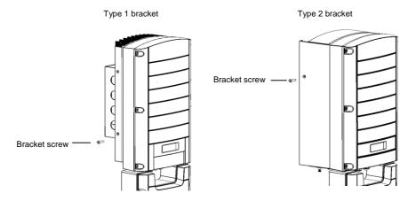
Figure 18: Inserting the bracket screws
