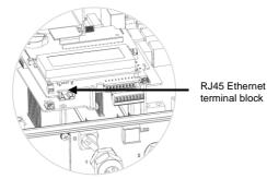
Figure 36: The RJ45 Ethernet connector
