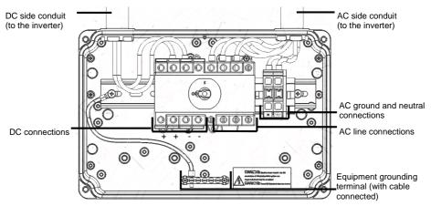
Figure 24: Inside the AC/DC Safety Switch for three phase inverters
