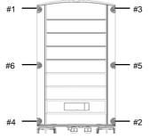
Figure 41: Tightening Order of the Screws
