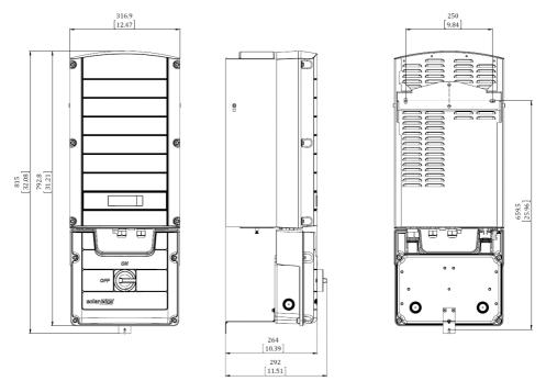
Figure 47: Single phase 7-11.4 kW inverter with brackets - front, side and rear views
