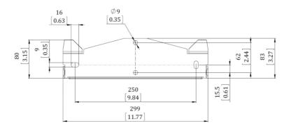
Figure 46: Inverter mounting bracket - Type 2
