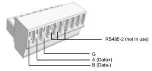
Figure 38: RS485/RS232 terminal block
