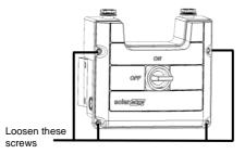
Figure 11: Opening the Safety Switch cover
