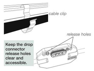
**b.** Dress any excess cabling in loops so that it does not contact the roof.
