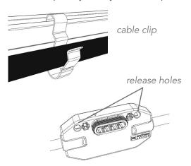
Keep the drop connector release holes clear and accessible.
