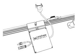
**b.** Mount the microinverters with the silver side facing up and the black side facing down.
