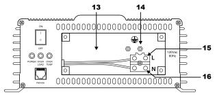
PST-1500 & PST-2000: FRONT - showing compartment containing AC output terminals for hardwiring.
