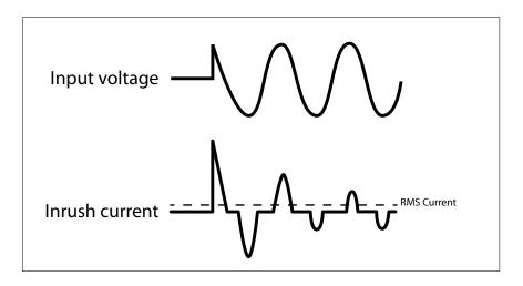
Fig 4.1: Inrush current in an SMPS
