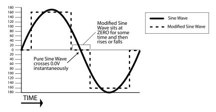
Fig. 2.1: Pure and Modified Sine Waveforms
