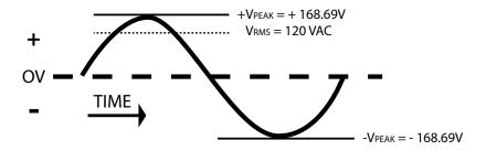
Fig. 5.1: 120 VAC, 60 Hz Pure Sine Waveform
