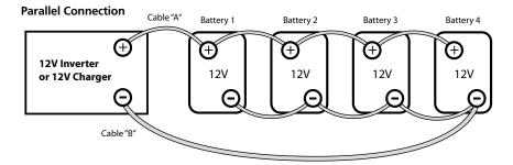
Fig 7.3: Parallel Connection
