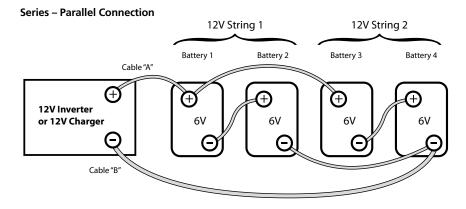
Fig. 7.4: Series-Parallel Connection
