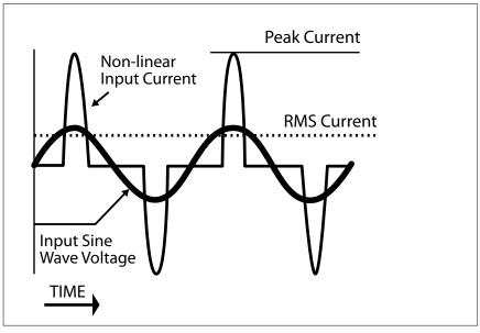
Fig. 4.2: High Crest Factor of current drawn by SMPS
