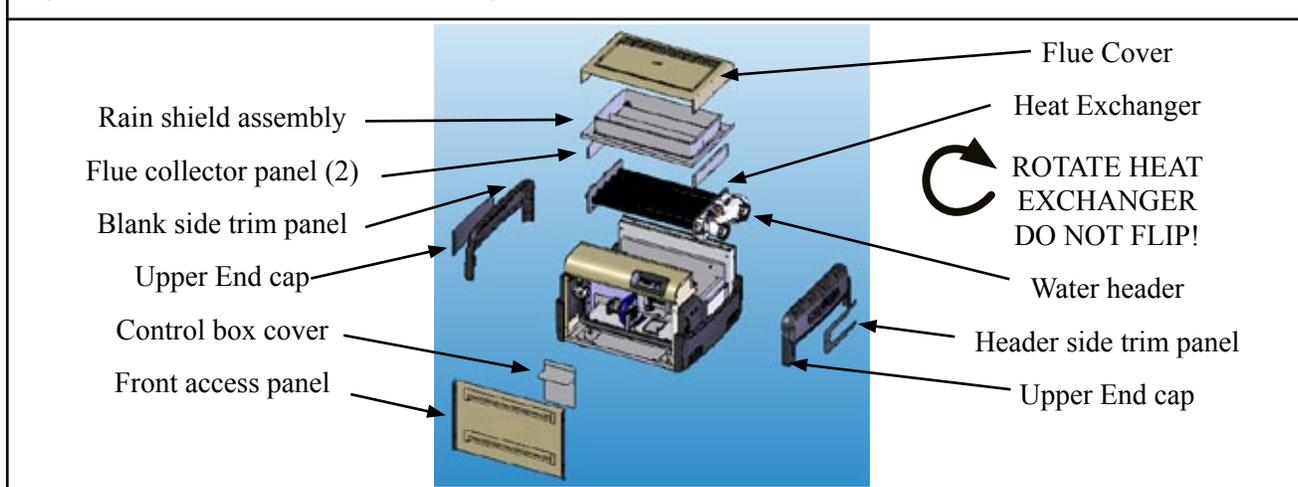
1. Before beginning, be aware that it is not necessary to remove the water header from the heat exchanger. When this procedure is complete, the water inlet will be located at the BACK of the heater. The water outlet will be located at the FRONT.
