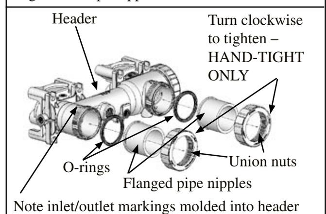
The built-in bypass inside the header will maintain proper flow through the heat exchanger if the flow rate is within the range for the heater. See Figure 20.
