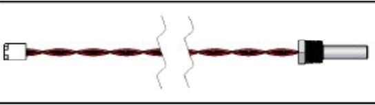
The thermistor monitors the return water temperature. See Figure 47. To replace the thermistor:
