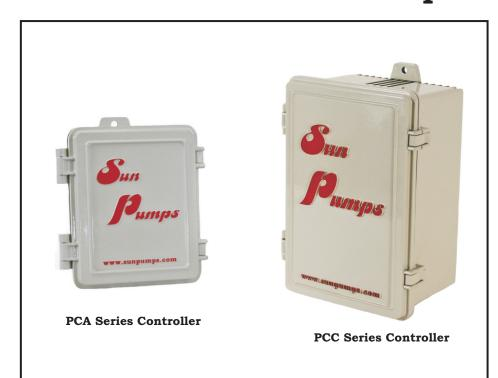
**SunPumps** PCA and PCC series pump controllers are high quality, micro-processor controlled DC power converters designed as the interface between a sensorless brushless DC powered pump and the power solar array. The main purpose of a PC series controller is for motor commutation, supply maximum power point tracking for the solar modules and provide protection for the controller.
