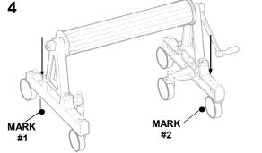
Using one of the two holes in the A-frame as a guide, make mark #1 on deck. With a 1/2" concrete drill bit, drill a 1 1/2" deep hole at mark #1. Complete steps 5 and 6 before continuing with step 4.
