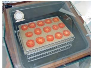
Turn one of the latches (located on the right hand side which seals the glass door) on the **SUN OVEN**® inward and set the glass on top leaving a gap between the black gasket and the glass to allow moisture to escape.
