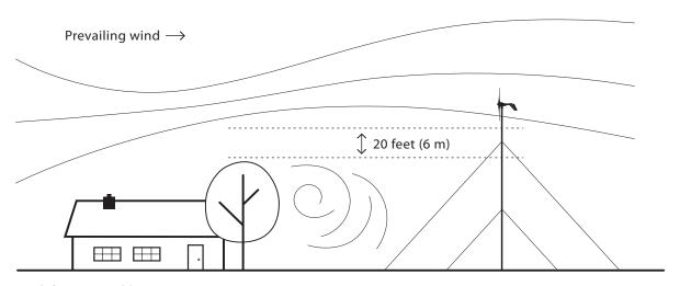
Fig. 2 Optimal AIR 30 location.
