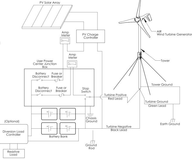
Fig. 11. Hybrid System with Solar Panels
