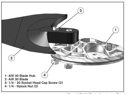
Fig. 1 AIR 30 Blade Attachment Detail.
