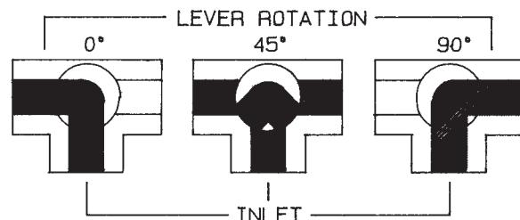
NOTE: Open port pressure must exceed Closed port pressure.
