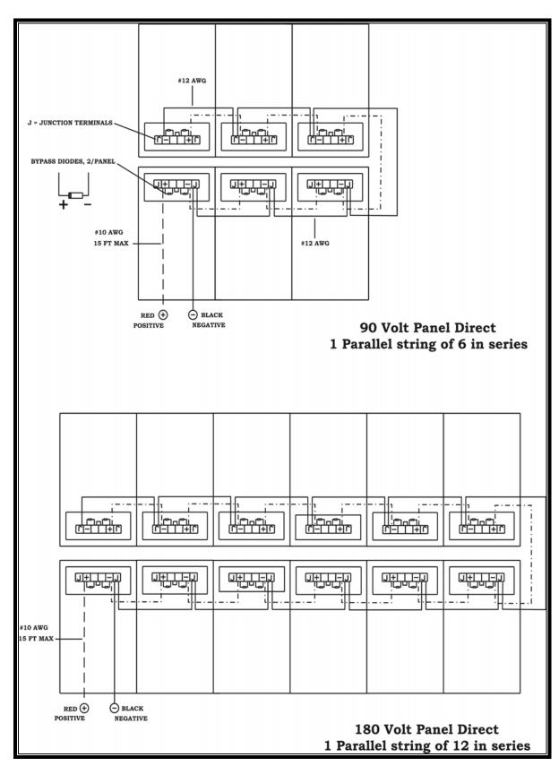
Figure 3 Cont. <u>Sample Solar Panel Wiring Diagram</u> (Generic)
