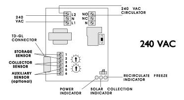
Adjust the <u>high limit</u> to the desired setting. The GL-30 will not allow the pump or fan to come on when the storage sensor temperature is higher than the storage high limit setting. Note that the
