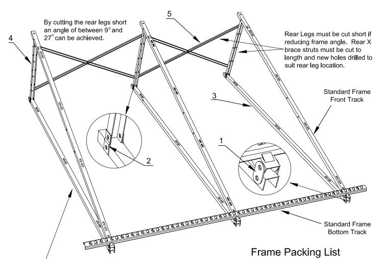
Attachment to roof may be via roof attachment straps, rubber pads or round feet, depending on roof surface. Such components are supplied with standard frame.
