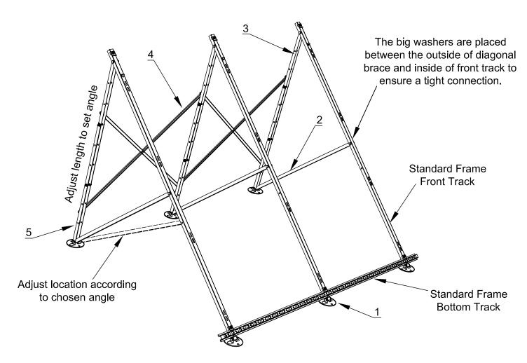
Nuts and bolts are already attached to the appropriate components
