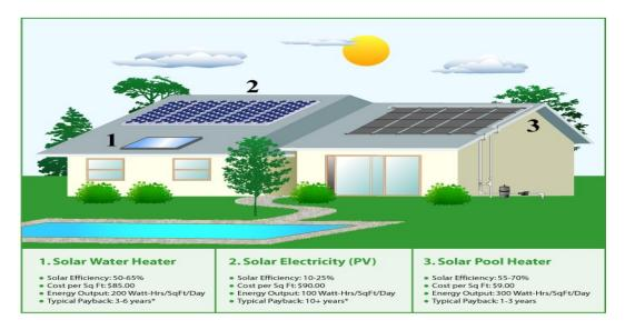
Solar Efficiency – This is the percentage of output of a solar panel compared to the average solar energy hitting the earth from the sun.
