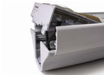
Figure 22: Removal of the Button Assembly
