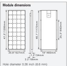
Hole diameter 0.26 inch (6.6 mm) Mounting hole dimensions are center to center
