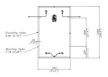
All measurements in mm. Inches in parentheses. Tolerances Length: ± 5mm (1/4") Width:  $\pm$  3mm (1/8")
