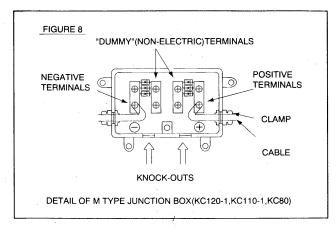
D. Read the enclosed instructions for routing wires through the knock-outs and clamps. (Figure 9)
