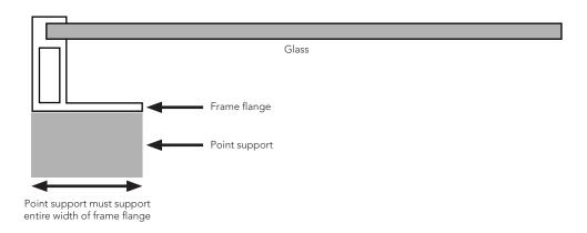
Figure 11: Location of point support in relation to the panel frame
