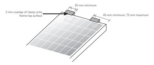
Figure 6: Clamping each panel without rails in direct contact with the panel
