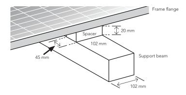
Figure 15: Spacer required between support beam and the frame flange
