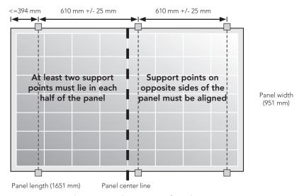
Figure 13: Required support locations for the 6 point option
