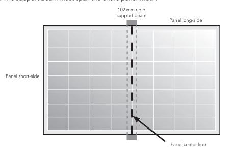
Figure 14: Required location of rigid support beam
