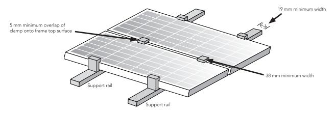
Figure 9: Permissible clamp arrangement for offset mounting
