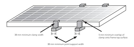
Figure 10: Point support and clamp requirements
