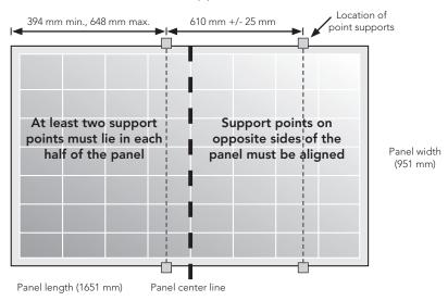
Figure 12: Required support locations for the 4 point option
