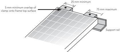
Figure 5: Clamping each panel frame individually
