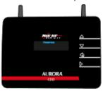
Choose the installation location of the CDD to configure the WiFi network and acquire the Micro Inverter. It is advisable NOT to fix the CDD to the wall in order to evaluate the placement based on the signal range.
