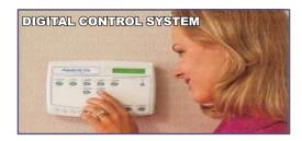
DIGITAL CONTROL SYSTEMS control the pool and spa water temperature from remote locations. Portable and fixed mount styles.
