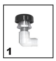
Seal all threads with Teflon tape (tape not included). Screw the vacuum breaker into the Elbow 90°
