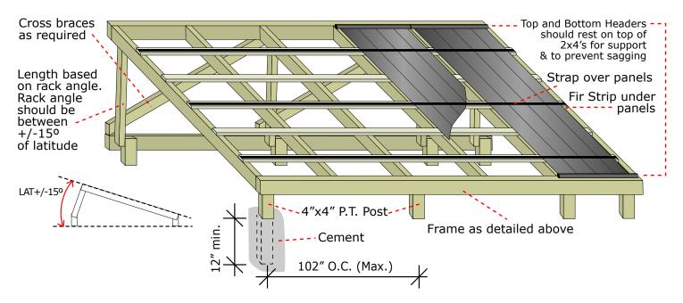
This design is generic in nature provided as an example of a typical rack layout and is not intended for all wind, snow and seismic conditions; engineering may be required based on site specific conditions and may require additional and/or alternative supports methods.
