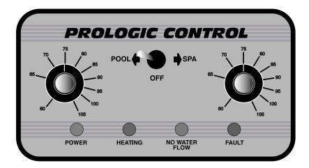
**TEMPERATURE CONTROLS:** The top Thermostat controls the pool temperature. The bottom Thermostat controls the spa temperature. If you do not have a spa you can use the two thermostats as a high and low temperature preset.
