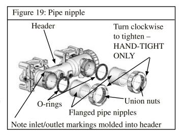
The built-in bypass inside the header will maintain proper flow through the heat exchanger if the flow rate is within the range for the heater. See Figure 20.
