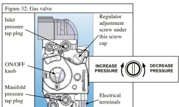
9. Remove the 1/8" pipe nipple and replace the 1/8" pipe plug. If proper pressure cannot be achieved by adjusting the gas valve regulator, the installer must contact the gas supplier and request that the inlet pressure to the heater be set to within the gas pressure range shown in Figure 33.
