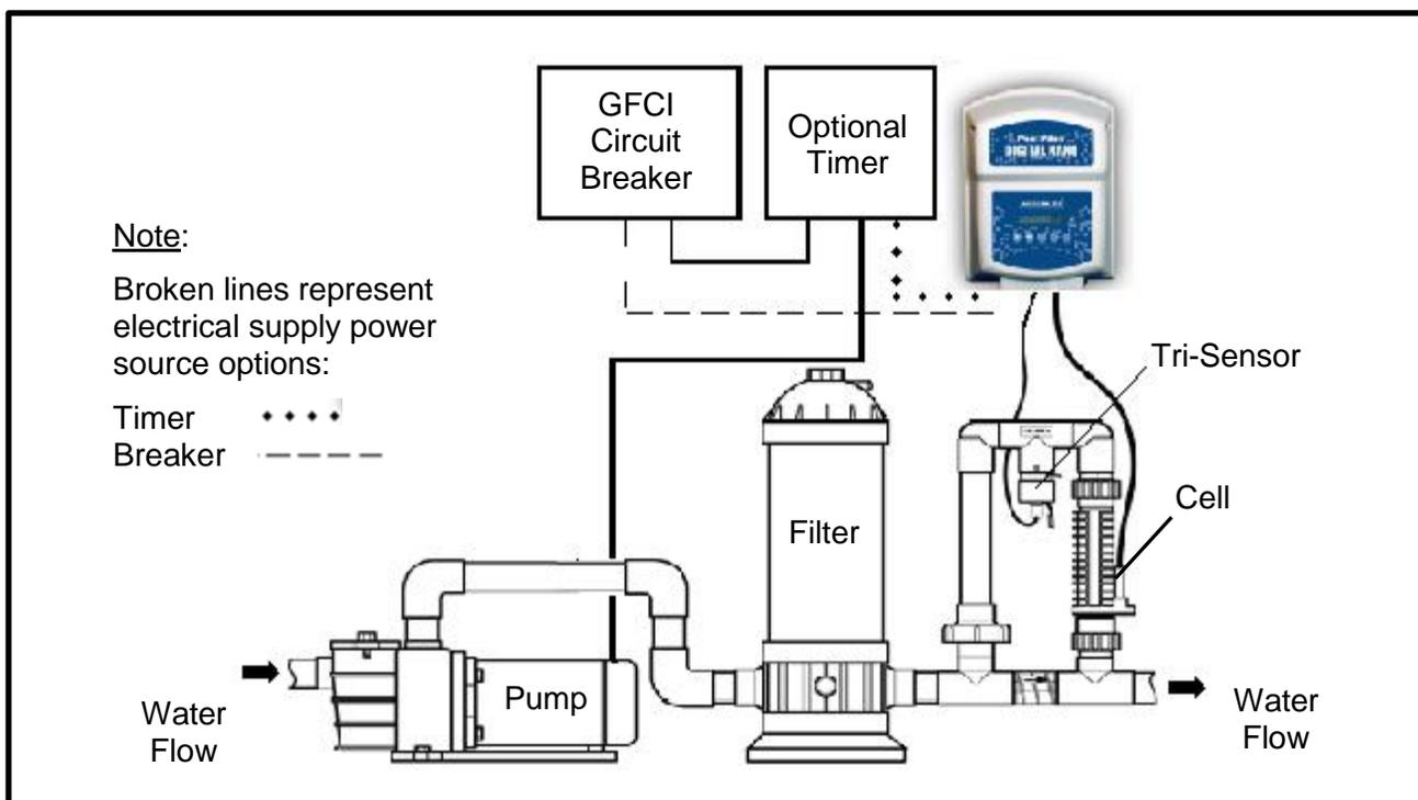
SHOWN WITH INLINE-CELL MANIFOLD ASSEMBLY (#75082)
