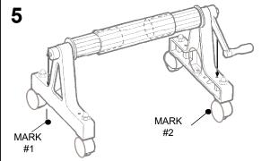
Using one of the two holes in the A-frame as a guide, make mark #1 on deck. With a 1/2" concrete drill bit, drill a 1 1/2" deep hole at mark #1. Complete steps 6 and 7 before continuing to the other side of the unit.
