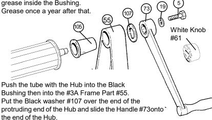
Put the washer #19 on the Bolt #5 and secure the Handle.
