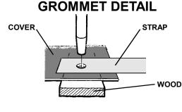
Position the blue strap on the cover. Make a hole, or cross cut through the strapping and the cover. Ensure that the hole in strapping is at least 2" from the end of the strap and that the hole in the cover is at least 2" from the end of the cover.
