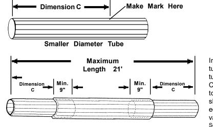
Insert smaller diameter tubes, into large diameter tube, up to the Dimension C mark, as shown. The total length of the tubes should be approximately equal to the corresponding value in column B. See example on reverse.
