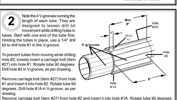
Drill hole #2A in V-groove, as per drawing. Do same on other end of tube set.
