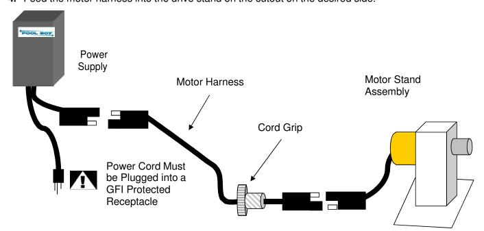
**5.** Install strain relief / cord grip on bracket in the base of the motor stand. Thread the motor harness through the bracket. Install the jamb nut and tighten.
