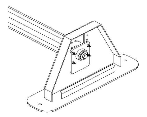
Using a 7/16 wrench, remove (4) mounting bolts.
