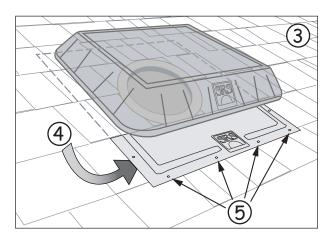
DO NOT OVER-TIGHTEN SCREWS, AS THIS MAY CAUSE UNIT BASE TO CRACK OVER TIME.
